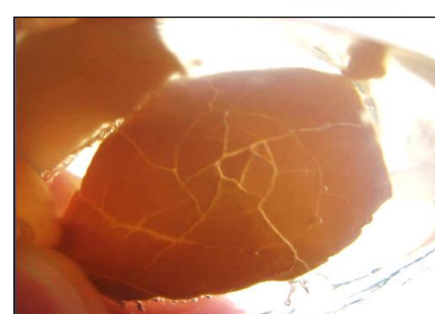
Egg shell after 7 Lithotripsy pulses
